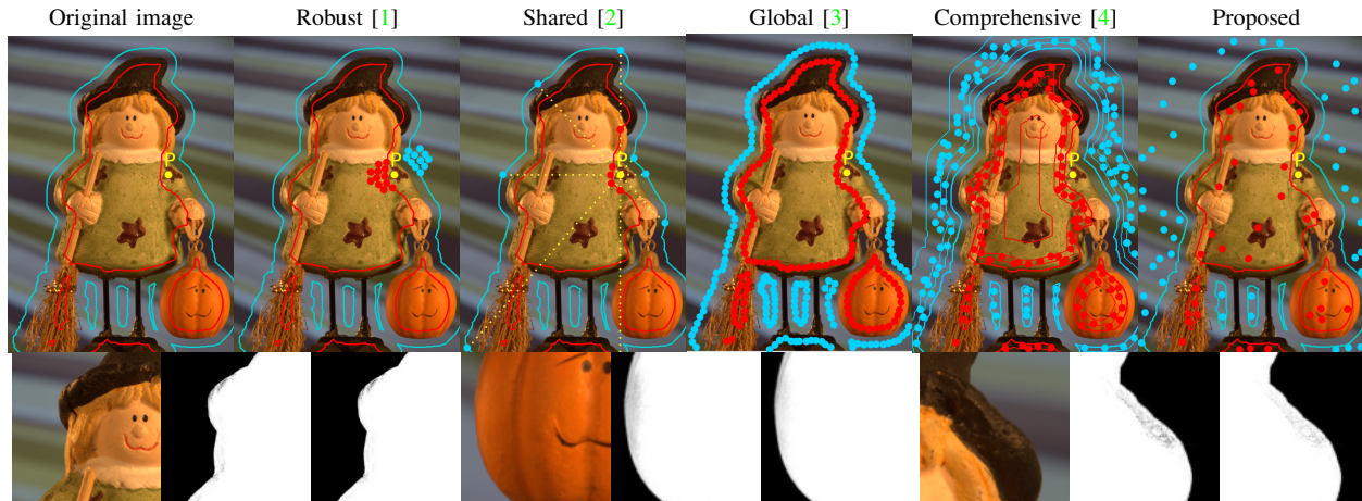
Fig. 1. Non-parametric sampling-based matting approaches. Top row: An input image and the representative samples gathered by the Robust [1], Shared [2], Global [3], Comprehensive [4], and the proposed Sparse Sampling based matting methods. The unknown pixel, the foreground and background samples are shown in yellow, red and blue colors, respectively. Bottom row: Comparison of the estimated alpha mattes by the suggested approach and the state-of-the-art Comprehensive Sampling matting method [4].
