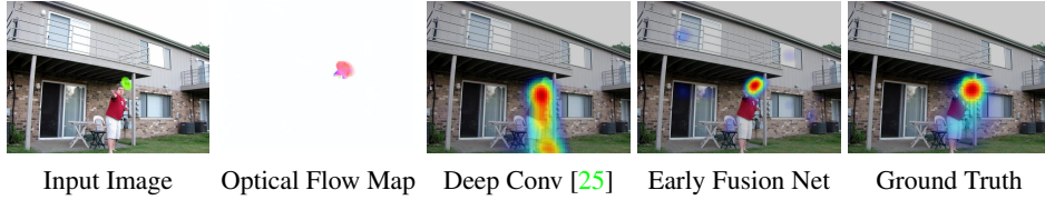
Figure 6. Transfer learning for static saliency estimation. Utilizing optical flow information estimated from static images can improve the prediction quality. Our finetuned Early Fusion Net produces a better saliency map than Deep Conv [25], a static deep saliency model.
