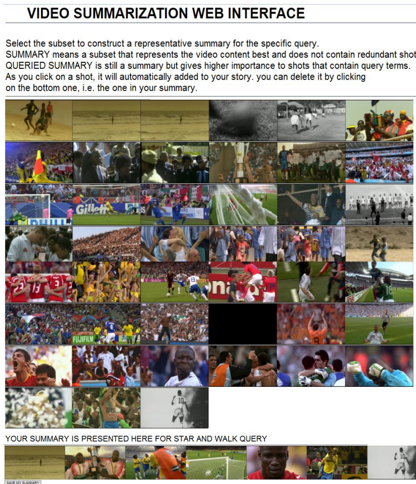
Fig. 5 A screenshot of the web interface used in obtaining ground truth query-specific summaries from human subjects. For a specific query for a video, the user selects fixed number of relevant shots as the summary. A sample human generated summary is shown at the bottom row.
