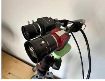
Fig. 1: A picture showing our data collection setup containing a PROPHESEE Gen4M event camera paired with an Allied Vision Alvium compact traditional CMOS camera.
